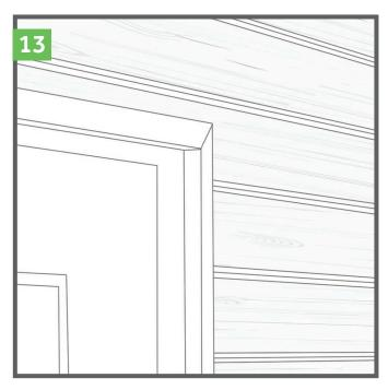
To finish your cladding, we recommend using any of our corner trim profiles. These are right angle profiles perfect for concealing corner joins and cladding ends.
