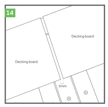
Where two boards meet lengthways, leave a 5mm gap to allow for thermal expansion.
